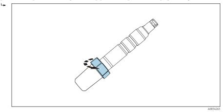
☑ 7 Releasing top part of protection cap by turning
