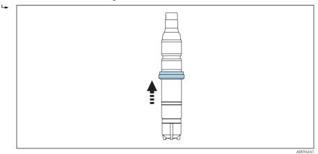
Islide the adapter (clamping ring) upwards from the membrane camp to the senor shaft and into the lower groove.
